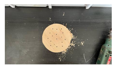
The first step is to prepare the base. To do this, we drill holes in the wooden base with a drill. Since we do not yet know exactly which pose our armature should take, we drill 10-20 holes at different distances in the base. The exact positions of the holes are secondary for now. The more holes you drill, the more flexible you are in the placement of the wire afterwards.
